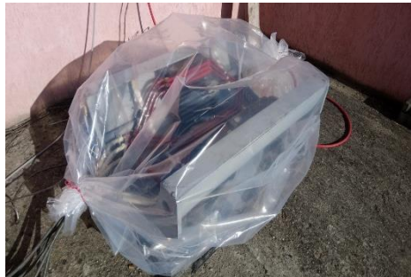
Fig.1. Insulation system subjected to overvoltage test in explosive mixtures
